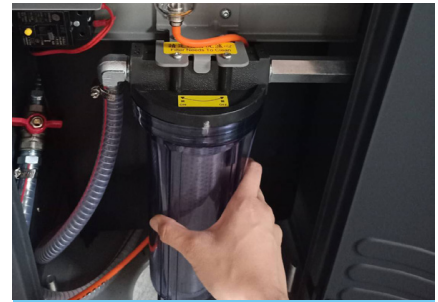
C. Remove the filter canister.
